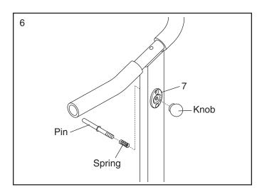
7. Insert the Frame Pin (45) through the Right Upright (9) into the hole in the Frame (41).
